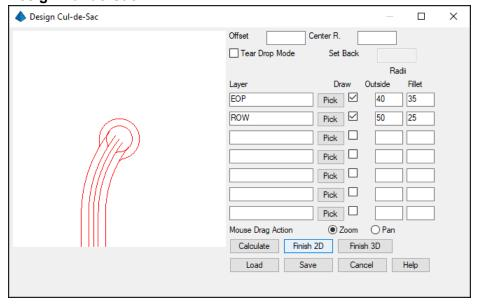
The *Design Cul-de-Sac* layout utility automates the process of creating geometry for Cul-de-Sacs. Similar to the Offsets and Intersection dialog box, this dialog box is where you set the desired geometric properties for the cul-de-sac.
