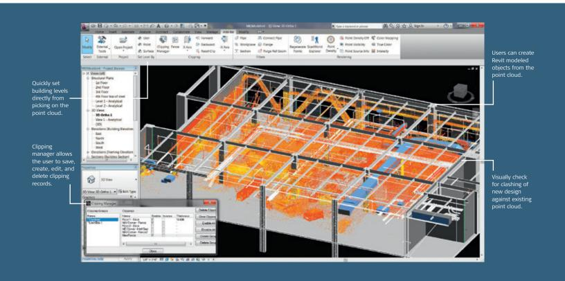
Leica CloudWorx 1.1 for Revit is a breakthrough plug-in for efficiently using rich as-built point cloud data, captured by laser scanners, directly within Revit for better BIM modeling of existing buildings. This is useful for a wide range of BIM activities including retrofit design, construction and operations, and lifecycle asset management of the building. It provides a virtual visit to the site within Revit with a complete view of the captured reality.
