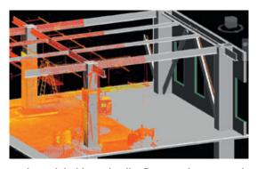
Revit model objects (walls, floors, columns, etc.) can be best-fit to the point clouds which provide accurate as built models.
